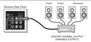
Connect the Pin cable from the TV's CENTER CHANNEL INPUT terminal to the surround amplifier's CENTER CHANNEL OUTPUT terminal.
